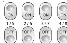
**2. ON/OFF Buttons.** There are 4 sets of ON/OFF buttons. They let you turn Modules 1 through 4 (or 5 through 8) on and off instantly by pressing either the ON or OFF button.
